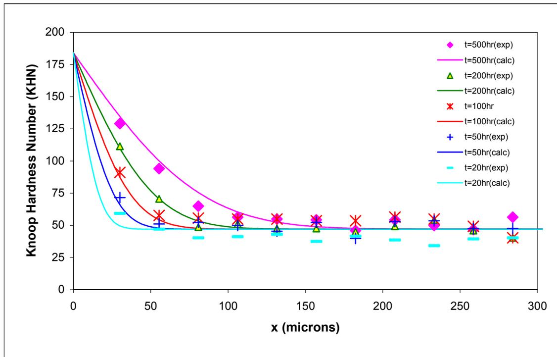
Figure 2 Microhardness profiles for samples annealed at 700°C
